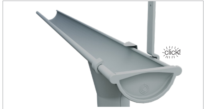
Press the gutter slightly together and twist the gutter down into the bracket lock at the rear edge.
